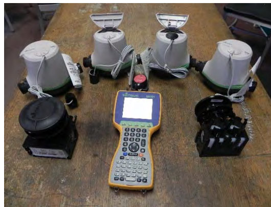
Commonly Used Radio Read Water Meters
