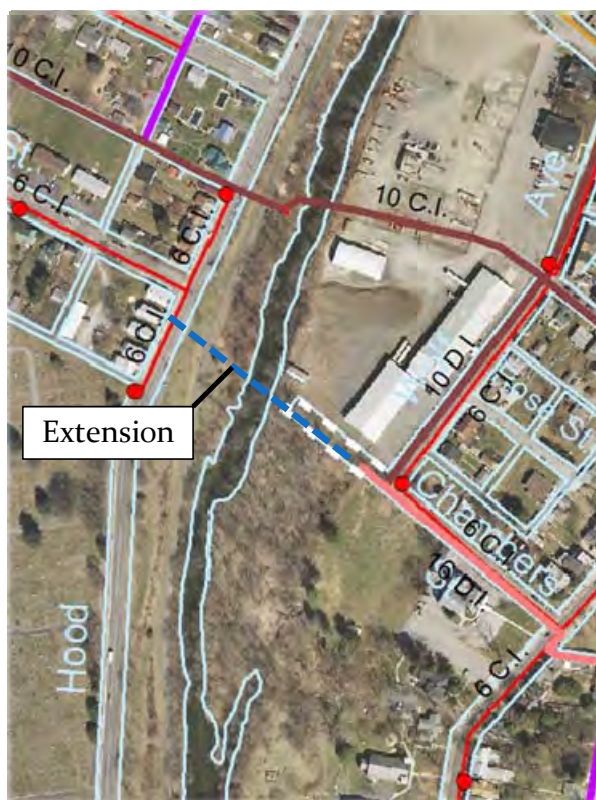
Chambers Street Water Main Extension
