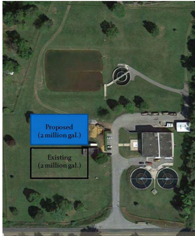
Water Treatment Plant Clearwell
